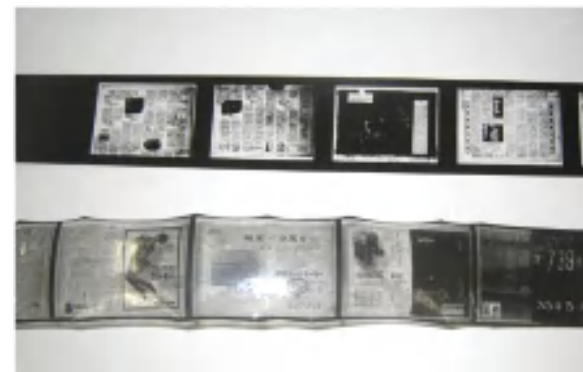
Polyester-based film in good condition (above) Deteriorated film (below)
